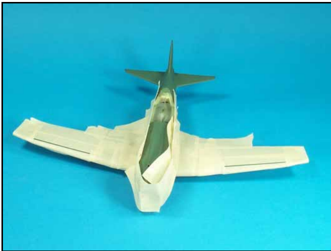
The final step in detail painting was to color the exposed inside areas of the forward wing flaps. Here again I used lots of masking tape to prevent any overspray.
