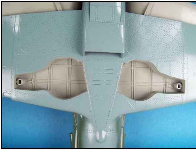
Wheel wells that have open areas are easily painted after the underside is painted. Note the sharp demarcation lines between the colors.
