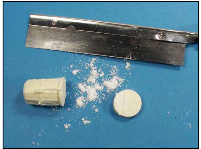
The pour plugs are best removed with a razor saw. The remaining plug can be wet sanded. Wear a dust mask when working with dry resin to prevent inhaling the dust.
