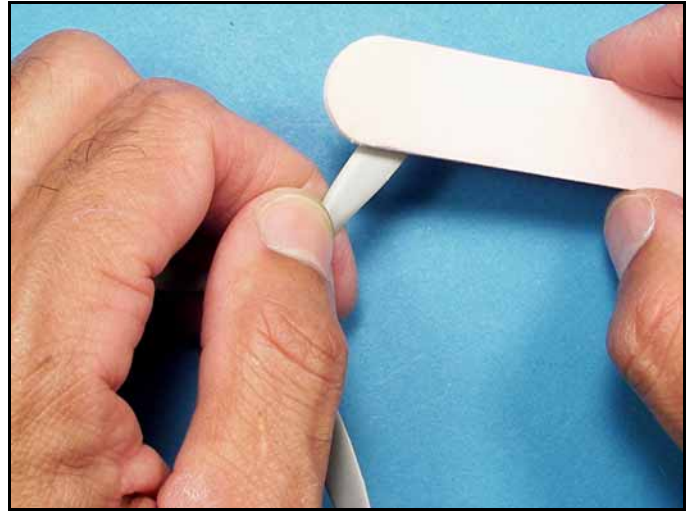
The edges of the blades sometimes have mold lines that need to be scraped off. Finish the props by wet sanding the surfaces with a sanding stick
