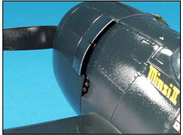
Another good example of drilled out exhausts. By using lots of drill bits with tiny changes in bit diameter you can achieve very thin plastic walls on exhausts.
