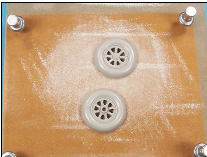
Flatten out the gluing surfaces for a tight fit. Just a few passes across the sandpaper will do the trick.
