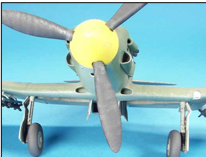
The air intakes look much better with actual screening. Small touches like adding screening and drilling out the exhausts add higher levels of visual realism to a scale model.
