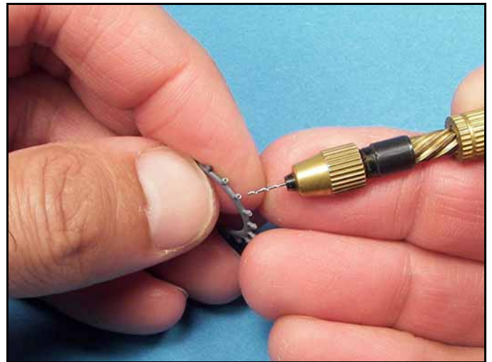
I used a number 79 (.0145 Inch) drill bit to drill tiny holes in the tabs so that the individual wiring for the spark plugs would have positive seating on the harness.
