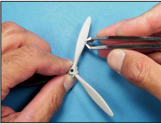
The first step in achieving good looking propellers is to carefully snip off the tree attachment points, and then sanding the area smooth with a sanding stick.
