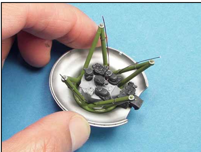
The engine control box and the engine brackets have been installed and I am now adding wiring.
